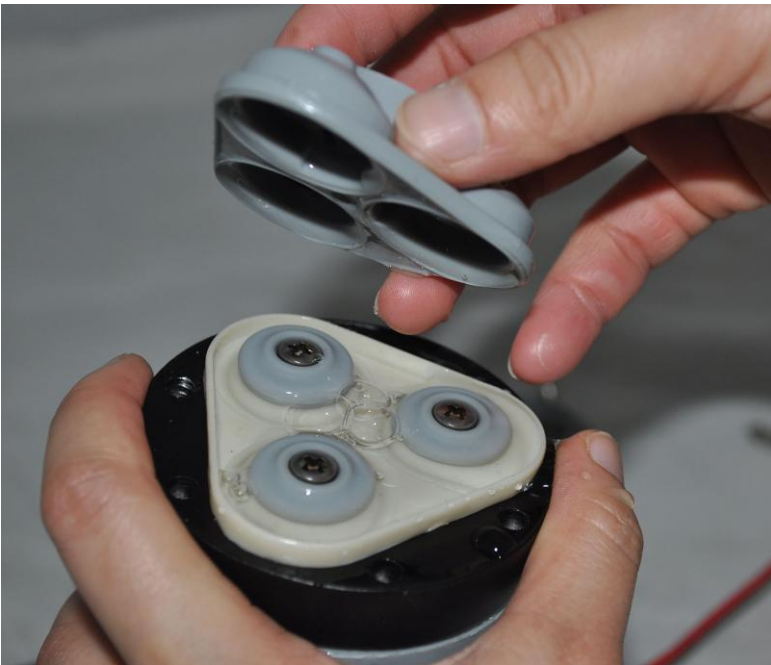
Replace the diaphragm seal and then assemble the pump cap back to the pump.
