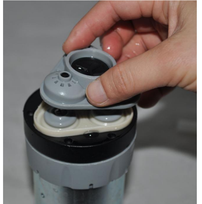
Replace the diaphragm seal and then assemble the pump cap back to the pump.
