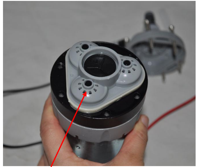
Unscrew the pump cap, see the diaphragm seal in the middle
